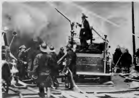
A FAR cry from the first pumping engine shown below is this modern piece of equipment that can pump 1000 gallons of water every minute and propel it hundreds of feet.
